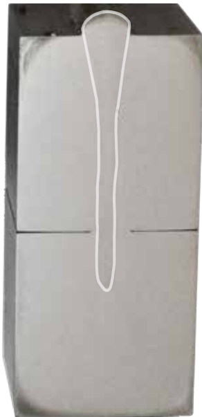
50 kW Power 1.5 inches (38 mm) Weld Depth
