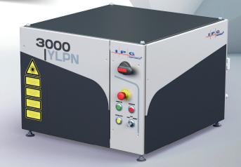
**YLPN-S Nanosecond Pulsed Fiber Lasers** offer variable pulse durations from 25 to 100 nanoseconds. The laser power can be adjusted in a wide range of pulse repetition rates independent of the pulse energy. Average output powers are up to 3 kW and pulse repetition rates vary from 2 to 300 kHz. Integrated beam switch option enables processing for multiple workstations in time or energy sharing modes.
