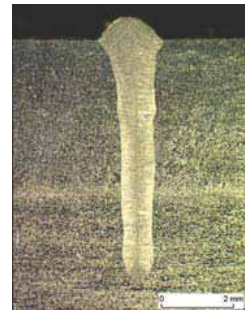
Fig. 5: Bead on plate weld, stainless steel, P= 6.9 kW, v=2m/min, gas Argon
