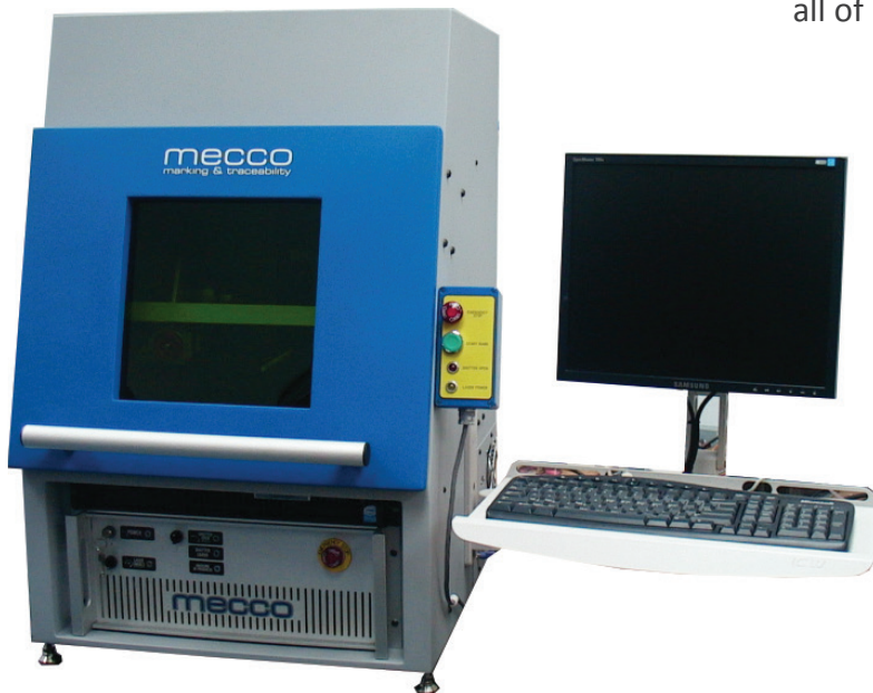
Figure 2: Mecco's Marking System Utilizing IPG's Fiber Laser
