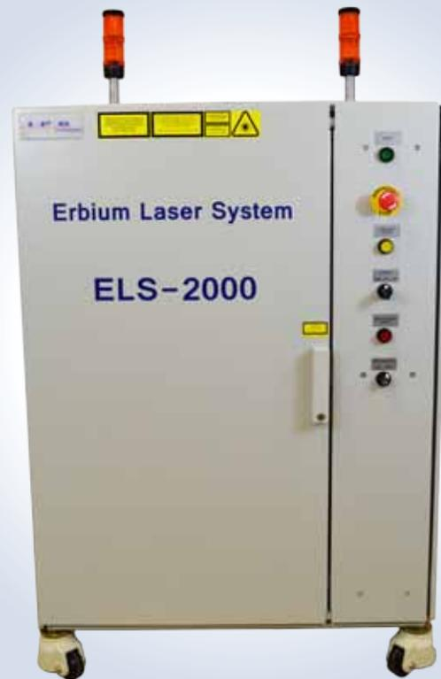
**IPG's new high power CW erbium fiber laser** has a central wavelength of 1567 nm and an output power of up to 2000 W. Featuring a power stability of  $\pm 2\%$  and a linewidth of  $<2$  nm. Available for research, materials processing and low loss power transmission applications, IPG's high power erbium lasers open up new exciting areas of applications development.
