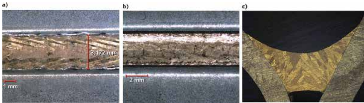
FIGURE 3. A comparison of single-spot (a) and trifocal (b) brazed seams that join steel with CuSi wire. An improved finish and suppression of edge roughness is evident in the trifocal brazing example. A cross-section (c) highlights the joint uniformity and quality obtainable with trifocal brazing.
