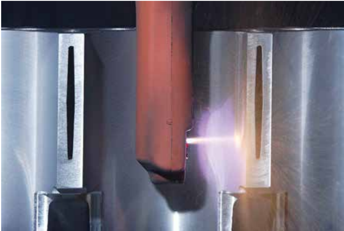
FIGURE 1. The cylindrical surface of a bore for an automobile engine is micromachined using a 2 kW single-mode fiber laser from IPG Photonics, then sprayed with plasma to create a hard coating that replaces conventional cylinder liners. Laser-machined microgrooves help the resulting coating to adhere to the cylinder. (Courtesy of IPG Photonics)
