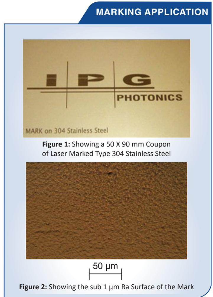
Using off-the-shelf scanning optics with a focal length of 163 mm, a focused laser spot size on the workpiece of  $\sim$ 50  $\mu$ m is readily achieved with the YLP laser. This gives an excellent depth of focus and hence any marking process will be tolerant to variations in the distance of the target from the lens. In this process, the actual line of oxide that is produced by laser heating on a stainless steel surface is larger than this focused spot size due to conduction effects.
