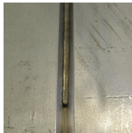
Examples of Wide-seam welding on Aluminum, Carbon Steel and Austenitic Stainless Steel
