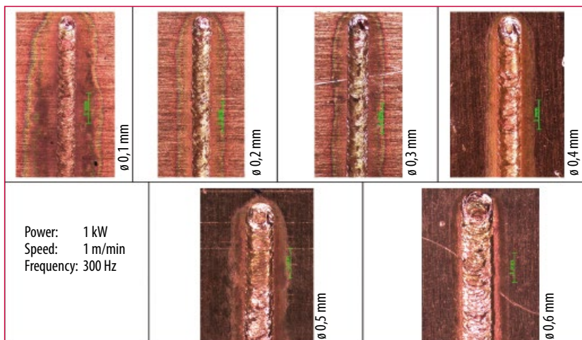
Fig. 5 Influence of the amplitude on the weld width and quality
