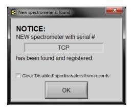
It means that the TCP/IP-connected device has been successfully added to the list of the spectrometers accessible through the MIIPS<sup>®</sup> 2.0 software interface.
