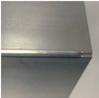
Corner weld on 6061-T6 aluminum (thickness 1.5 mm)
