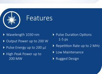
IPG Photonics NEW **YLPP-200-1-200** hybrid-fiber picosecond laser provides high peak power with scalable average output power of 200 W and customer selected pulse durations in the range of 1 to 5 ps at full operational repetition rate range of 50-2000 kHz.
