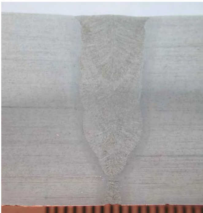
Figure 9. Laser root/GMAW fill weld in X100 plate
