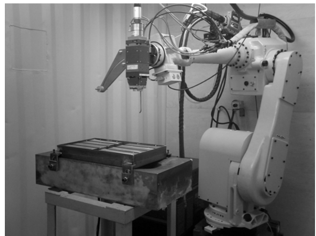
Figure 3. Experimental set-up for welding of pipe steel in the flat position.
