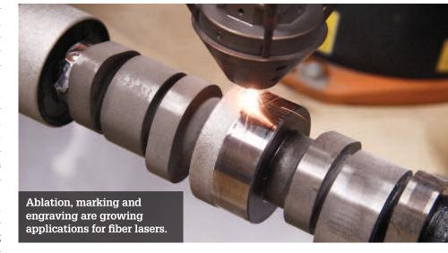
or remove oxide layers and coatings prior to welding. "It's quicker and produces less waste," notes Samson.
