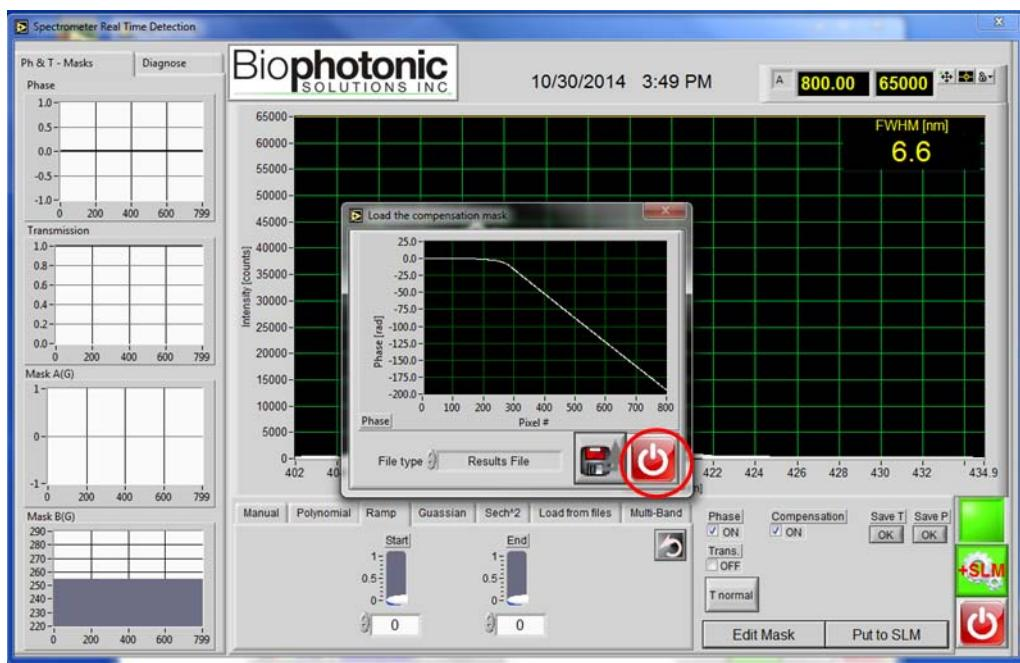
At this point, the user can choose to either apply the phase compensation mask alone or add some mask on top of it using one of the tab functions; e.g., using the “Polynomial” tab.
