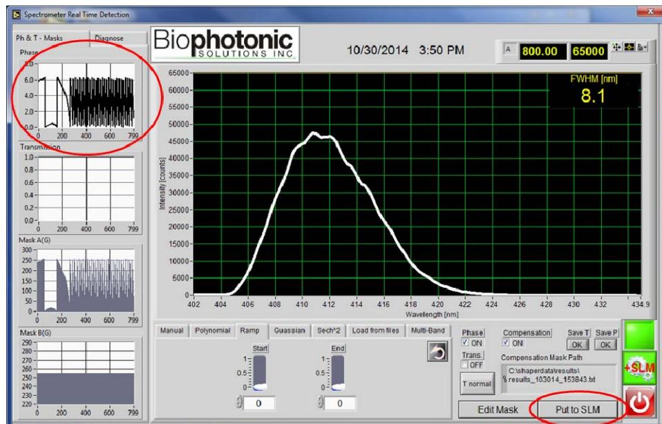
Note that the plotted phase profile will change to reflect the offset and wrapping that fit the calculated mask into the liquid-crystal retardance range. Again, one should see the effect of the applied mask on the monitored spectrum (if applicable).
