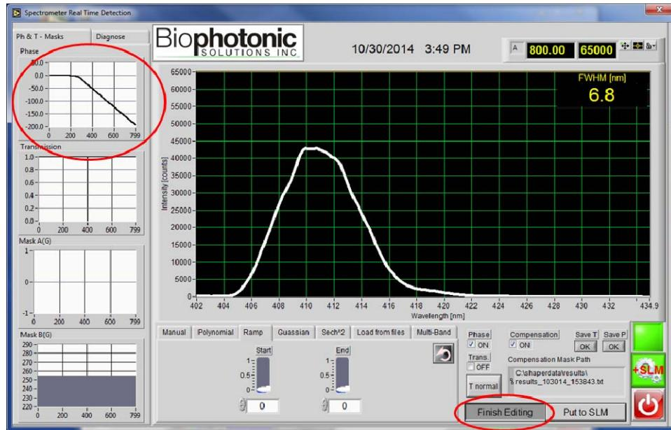
Press the “Put to SLM” button to write and activate the calculated mask.
