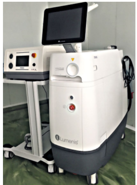
Fig. 2 | Comparison of lasers for lithotripsy. An air-cooled, tabletop, quasi-continuous-wave thulium fibre laser with 50 W average power, 500 W peak power, and pulse rates up to 2000 Hz is shown on the left. A high-power, 120 W holmium:yttrium–aluminium–garnet (YAG) laser, capable of pulse rates up to 80 Hz, for stone dusting applications is on the right.
