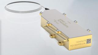
IPG Photonics **PLD-224-200-970-CHL** fiber-coupled packaged diodes provide 180 W of output power at 20 Amps. The PLD-224 features a 200 µm fiber core diameter and a 970 nm center wavelength. Wavelength stabilization and dichroic options are available.
