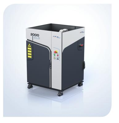
**IPG's new high power CW erbium fiber laser** has a central wavelength of 1567 nm and an output power of up to 2000 W. Featuring a power stability of  $\pm 2\%$  and a linewidth of < 2 nm. Available for research, materials processing and low loss power transmission applications, IPG's high power erbium lasers open up new exciting areas of applications development.
