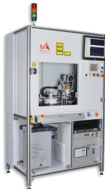
Fig. 1 The industrial laser systems from Limo are the “heart” of Medicom’s welding lasers, which are used by well-known automotive suppliers for the reliable production of pressure- and liquid-tight plastic fuel filter enclosures. (Source: Medicom)
