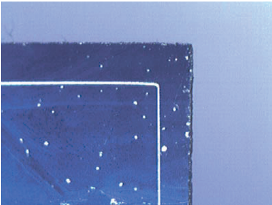
Edge isolation groove scribed with a 20W YLP laser
