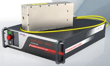
**NEW YLPP-200-1-200** hybrid-fiber picosecond laser provides high peak power with scalable average output power of 200 W and customer selected pulse durations in the range of 1 to 5 ps at full operational repetition rate range of 50-2000 kHz.
