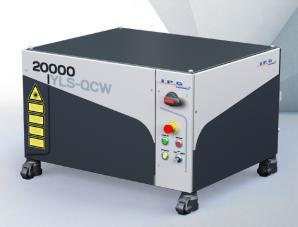
The **YLS-2000/20000-QCW** Quasi-CW fiber laser delivers high peak power of 20 kW, pulse durations of 0.2-10 ms and a maximum pulse energy of 200 J at repetition rate up to 2 kHz. The YLS-2000/20000-QCW laser is well suited to drilling and cutting applications within the aerospace industry, where percussion drilling, trepanning and fine cut features are often required.
