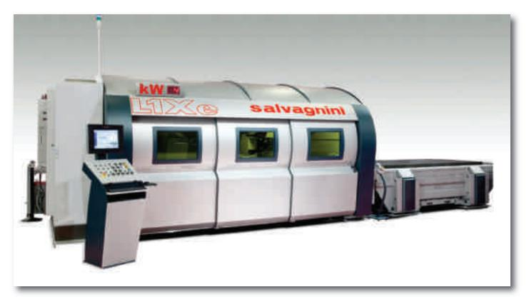
A Salvagnini L1Xe fibre laser profiling centre has helped Ashford-based Kent Metal Developments (KMD) replace two eight-year-old CO<sub>2</sub> lasers, a move that has led to a considerable cut in energy consumption without any loss of capacity thanks to the new machine's impressive speed of cut, automation and output capability.
